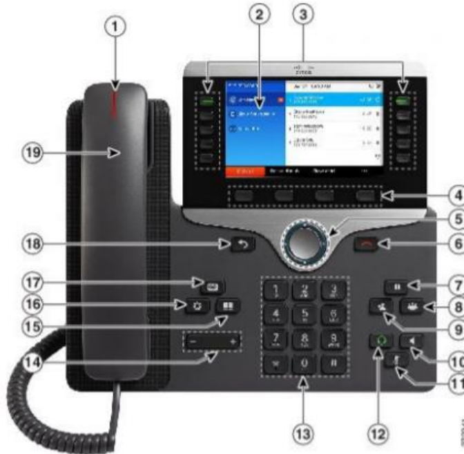
Figure 2 – Cisco CP-8851 hardware layout
